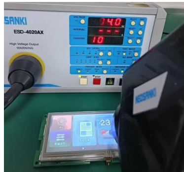
3.1 Electrostatic discharge test
